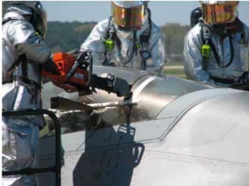
Cutting the pilot out of the locked cockpit of an F-22.
