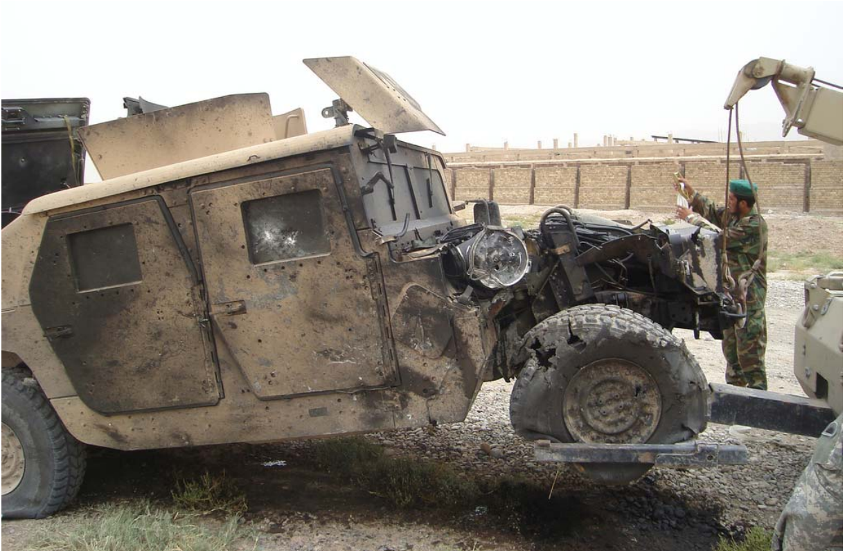
Hit By Vehicle Born IED: Kandahar: [Thanks to Kevin Ramirez, CCCO, who sent this in.]
