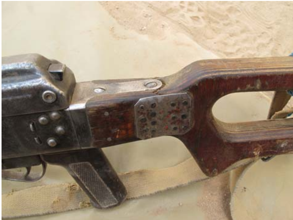
A machine gun with a cracked stock and a jury-rigged repair. C.J. Chivers for The New York Times
